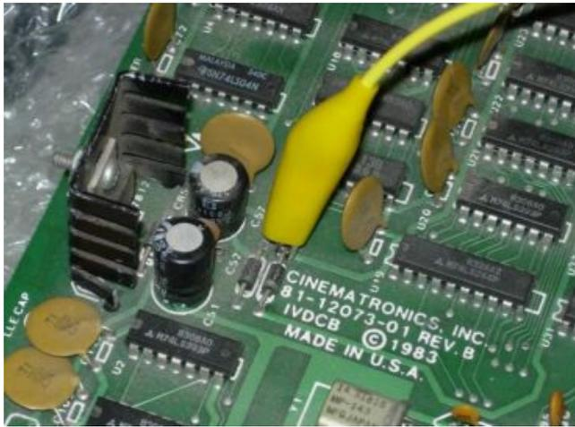
(A good connection point is the anode of diode CR6, middle left of the board, or the positive leg of any disc capacitor.)
