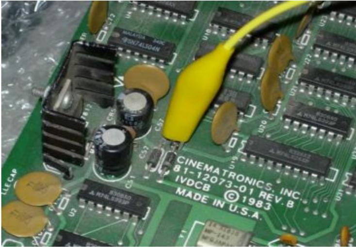
(A good connection point is the anode of diode CR6, middle left of the board, or the positive leg of any disc capacitor.)
